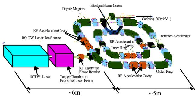
Compact Heavy-Ion (Carbon Ion) Synchrotron
