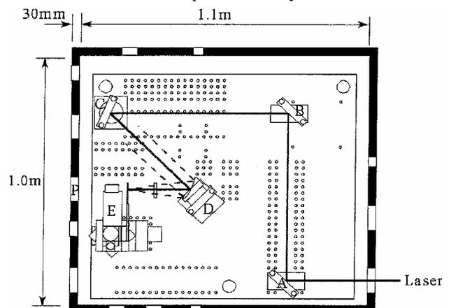
Fig. 4 Optics of the final focusing at the foil target in the vacuum chamber.
