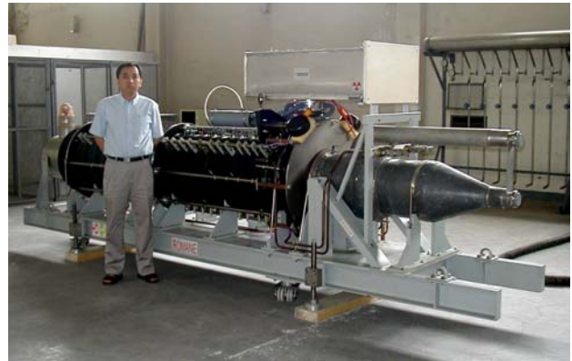
Fig. 7 The 352.2MHz/1.2MW CW klystron from CERN has been moved to IHEP, Beijing.
