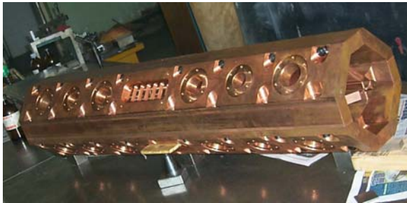
Fig. 5 The copper cold-model RFQ cavity of 1.2 meter long.
