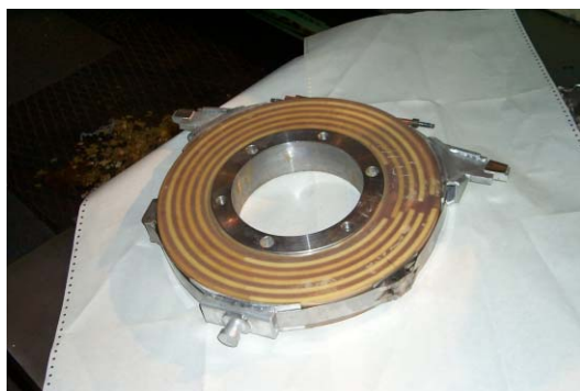
Figure 3: A built coil that will form, together to the others 19, the BRIC solenoid.
