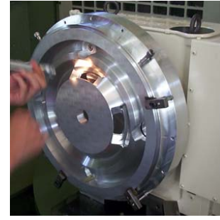
Figure 6: Trial machining of the aluminum model on a machining-centre
