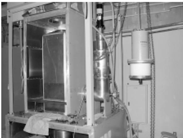
Fig.2 Photograph of a new test bench for testing a 1.4 MW RF tube (Siemens RS2074SK).
