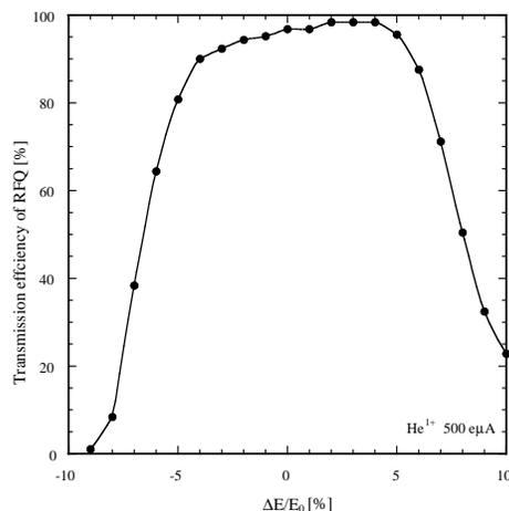
Fig.1 Dependence of transmission efficiency of RFQ on the input energy (7.2~8.8 keV/n). Only an acceleration voltage for the source terminal was changed. The center energy (0%) in the X-axis corresponds to 8 keV/n ( $E_0$ ).
