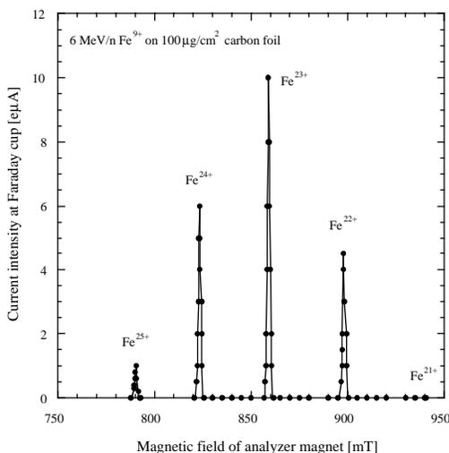
Fig.3 Charge distribution of Fe ions after stripping at  $100 \mu\text{g}/\text{cm}^2$  carbon foil with impact of  $6 \text{ MeV}/n \text{ Fe}^{9+}$  ions. The fraction of  $\text{Fe}^{23+}$  is largest, and is usually used for the injection into the ring.
