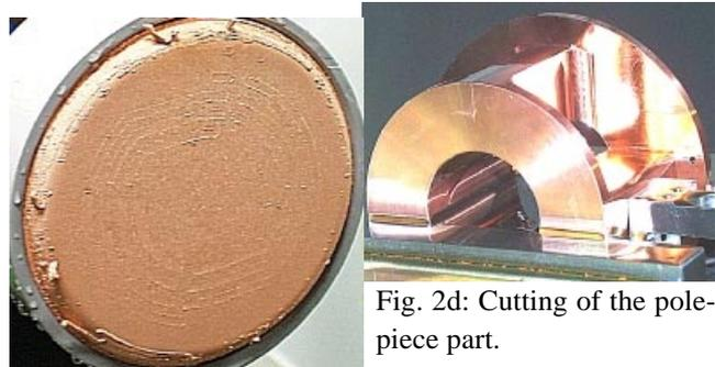
Fig. 2c: PR electroformed surface.
