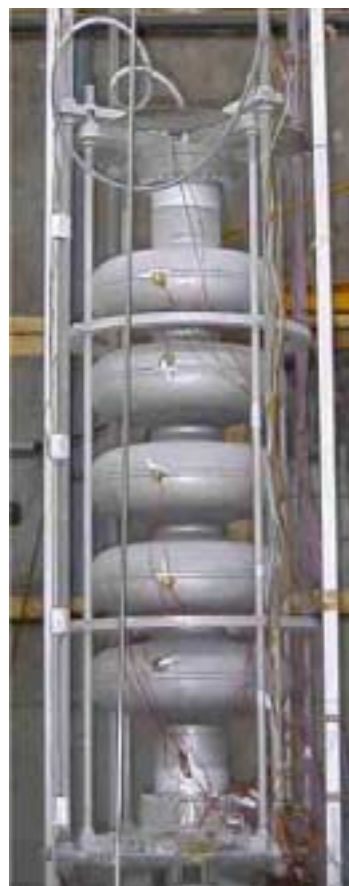
Fig. 3 A 5-cell cavity of \beta=0.89
