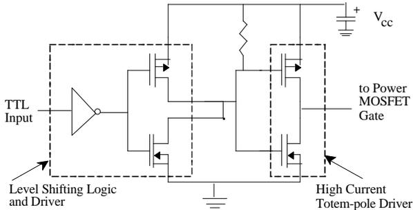
Fig. 1 Simplified Schematic of MOSFET Drive Circuit
