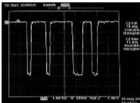
Fig. 7 Four Pulse Burst at 10 kV into 50 Ω Load
