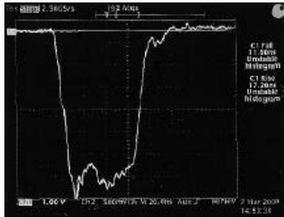
Figure 8: Output voltage versus time from experimental data (with a 12.5 stalk).
