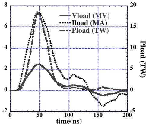
Fig. 3 Outer diode ring (bottom MITL) waveforms.
