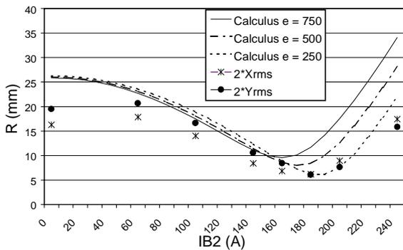
figure 4: beam imaging on the final beam stop (BS), with the B2 coil variation.
