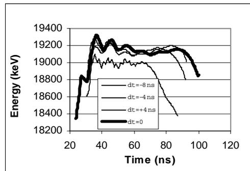
Figure 4 : Variation of duration of beam with synchronization of H.V. generators
