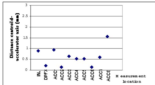
Figure 5 : Positon of the beam along the accelerator
