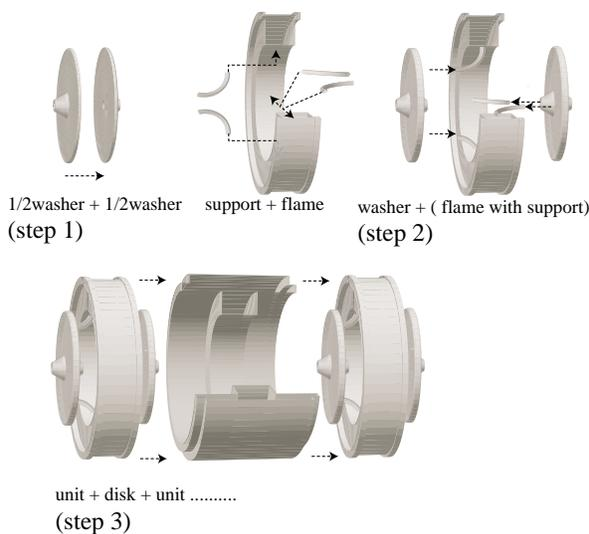
Figure 1: Fabrication steps of the biperiodic L-support DAW
