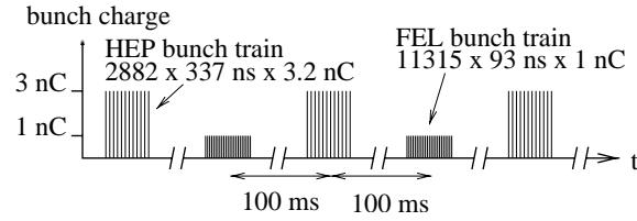
Figure 2: HEP and FEL beam pulse structure
