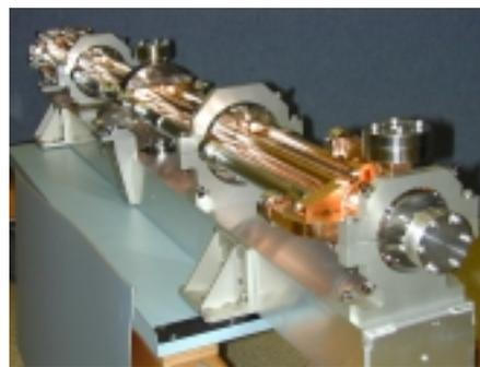
Figure 1: RDDS1 section installed on a strongback. Properly chosen, three arcs in the RDDS design optimized the shunt impedance, Q value and minimized the ratio of peak surface to average accelerating electrical field. Also, the modified HOM coupling slots reduced the leakage of the fundamental mode by a factor of two. Compared to DDS, the overall improvement in shunt impedance for RDDS1 is about 19%.
