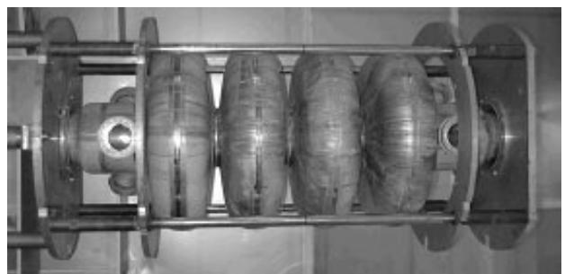
Figure 5: The prototype 4-cell  $\beta=0.7$  cavity
