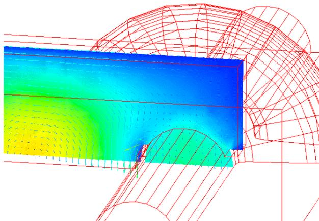
Fig. 3. Electric and magnetic fields in the feed waveguide and at the coupler aperture of the structure shown in Figure 1. Arrows show magnetic field and spectral plot shows the electric field.
