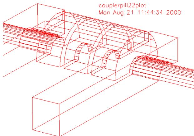
Fig. 2. Upper half of waveguide cavity input couplers with dual slots for a three-cell S-band structure. Coupling slots are on the wall of the end cavities.
