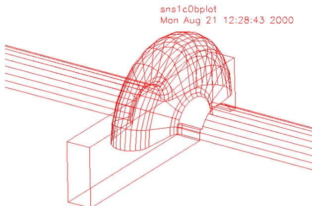
Fig. 1: Half structure of waveguide cavity input coupler with dual slots on the beam pipe. Coupling slots are on the beam pipe.
