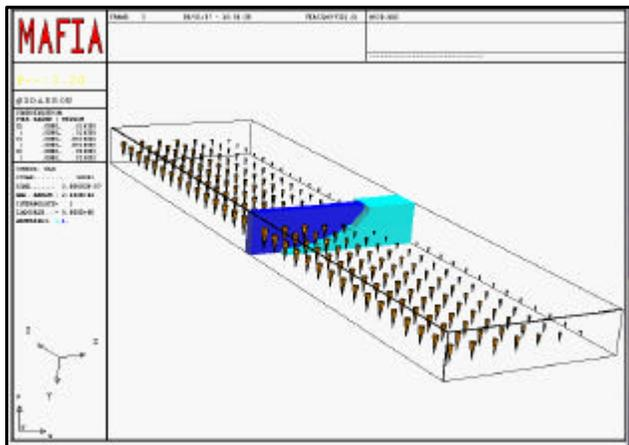
Figure 6: CESR window electric fields as calculated by MAFIA
