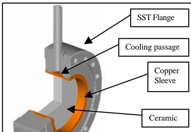
Figure 2: Section showing ceramic, copper, and SST
