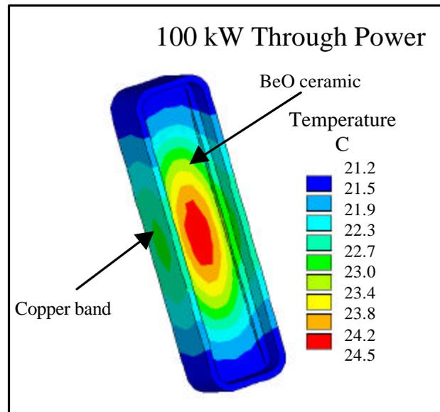
Figure 4: Temperature profile through the JLAB window for 100 kW of thru power
