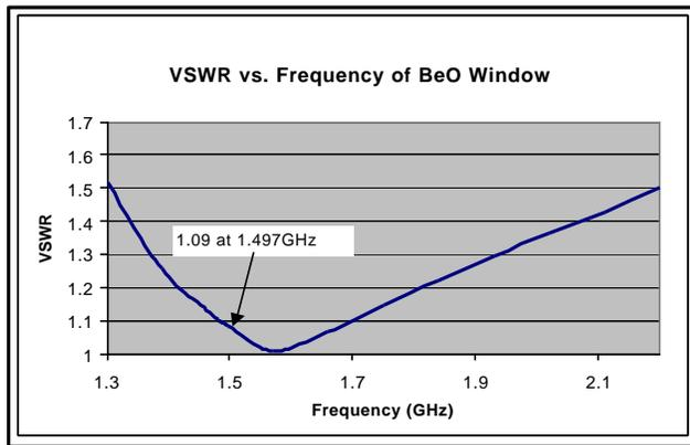
Figure 3: VSWR vs Frequency for the JLAB BeO Window
