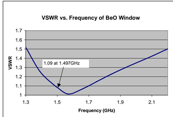
Figure 3, VSWR for required frequency range
