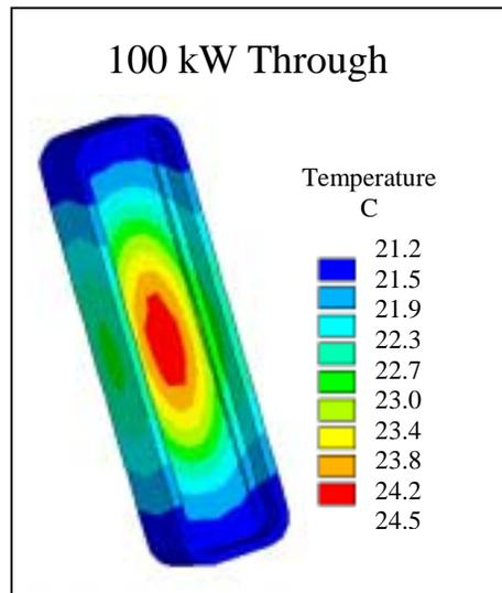
Figure 4, Window temperature contours
