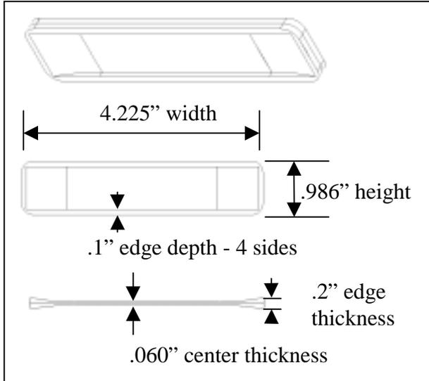
Figure 2, Window design parameters
