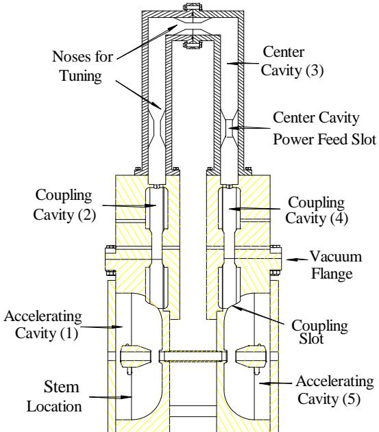
Figure 1. Drawing of Bridge Coupler Cross Section.
