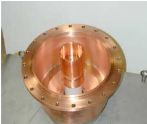
Figure 4: Tubular ceramic in a coaxial housing
