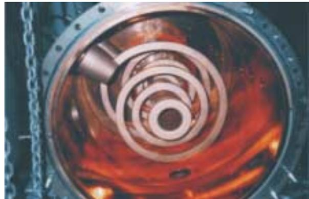
Figure 5: View inside 36 MHz 1.4 MeV/u rebuncher
