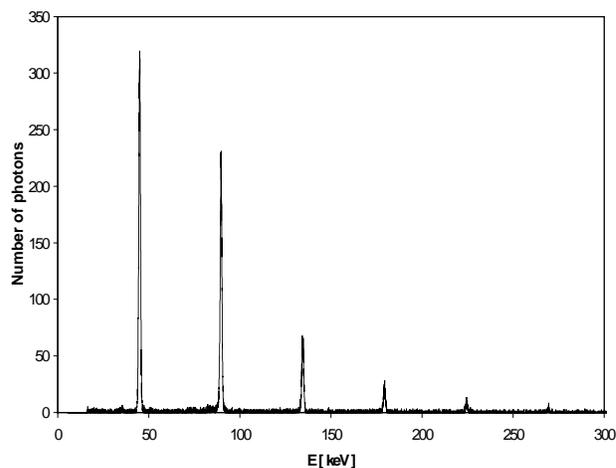
Figure 3: Typical spectrum from a symmetrically-cut crystal
