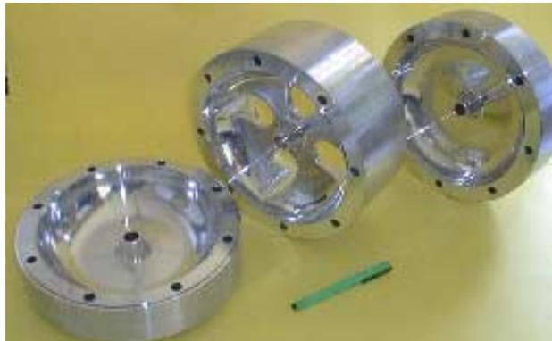
Fig. 6. Trispal cavity cold model. The central piece (with holes) can be removed for 1-cell measurements.
