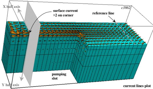
Figure 2: Surface currents deviated by a pumping slot.
