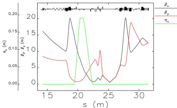
Figure 2: Typical Twiss parameters in the chicane region.
