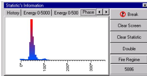
Fig.6. Equilibrium phase distribution at the moment of emission in the resonant discharge.
