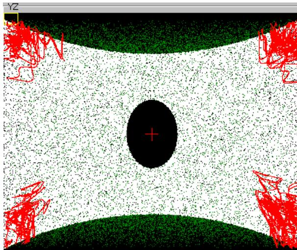
Fig.8. The electron trajectories in the non-resonant multipaction.
