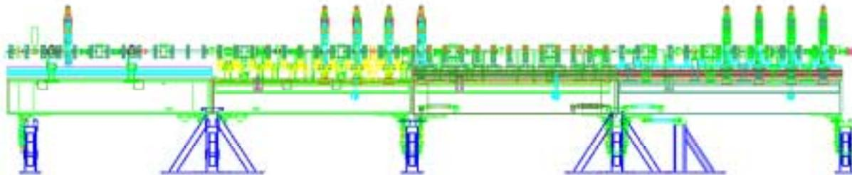
**Figure 1 Overall Layout of the Beam Halo Experiment on LEDA. The transport line consists of 52 quadrupoles between the LEDA RFQ and the HEBT/beam stop. The first four quadrupoles are used to create a controlled mismatch from the RFQ. A series of nine dual-axis, high dynamic-range wire/scrapper scanners will be used to measure halo properties.**
