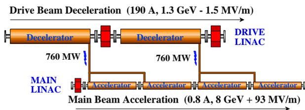
Figure 1: The Basic Concept of Two-Beam Acceleration
