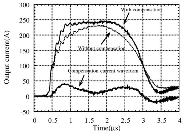
Figure 4: Output current waveforms with and without compensation, and the compensation current waveform.
