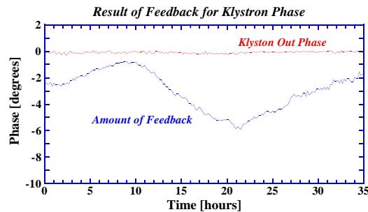
Figure 7: Stabilized klystron phase and feed-back amount.
