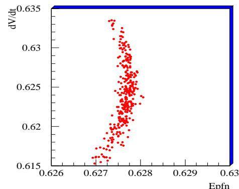
Figure 5: x and y axe show  $E_{PFN}$  and  $dV/dt$  respectively. Data were taken with fully optimized feed-forward controlled deQ.
