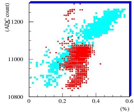
Figure 4: x and y axe show the momentum jitter,  $\Delta P/P$  and amplitude of AC 200V line respectively.
