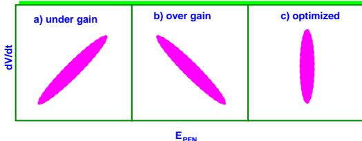
Figure 3: Schematic  $dV/dt$  -  $E_{PFN}$  plots for three cases; a) under gain, b) over gain, and c) optimized.
