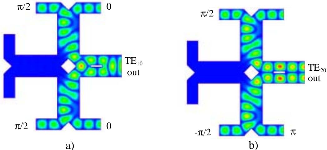
Figure 2: Example Cross Potent Launcher with simulated electric field plots illustrating launching a) TE<sub>10</sub> and b) TE<sub>20</sub> in the right overmoded rectangular port with the indicated relative phases for four equal amplitude inputs. Alternate phasings of the inputs send the power to either of the left ports.
