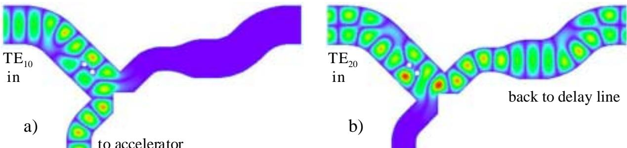
Figure 3: Extractor with simulated electric field plots illustrating a) extraction of the  $TE_{10}$  mode and b) passing the  $TE_{20}$  mode. For the latter, a “jog converter” attached to the through port after a width taper restores the mode and brings the port back in line with the delay line. Power flow is from the left port.
