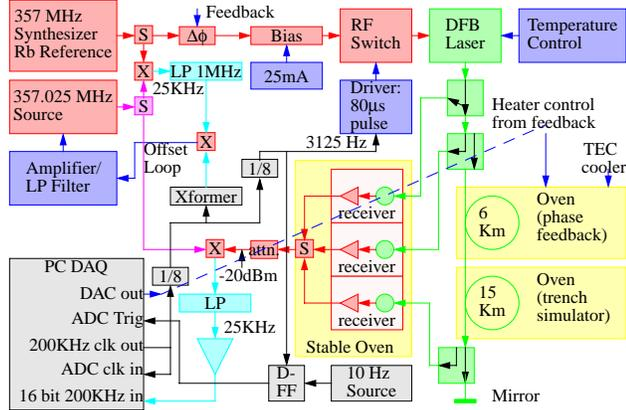
Figure 4: Phase Stabilization Test System
