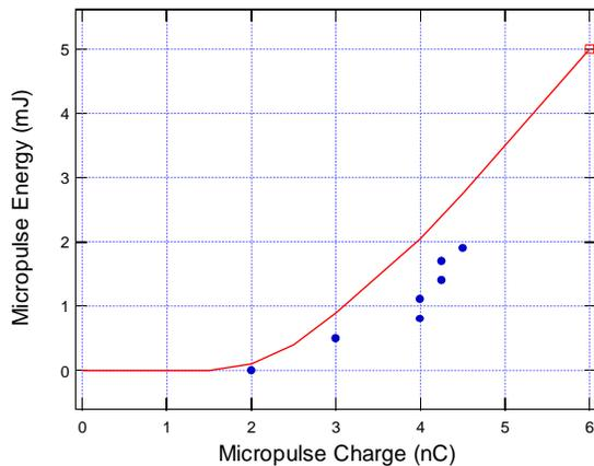
Figure 5: Plots of micropulse energy versus micropulse charge. The line is estimates based on FELEX simulation (square) and the circles are experimental measurements.
