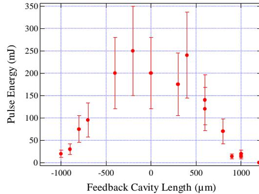
Figure 6: Plots of macropulse energy versus optical feedback cavity length.
