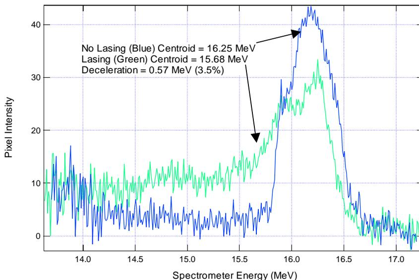
Figure 6. Electron beam energy exhibits a 3.5% mean energy shift, indicating an FEL efficiency of 3.5% as measured with the electron energy spectrometer.
