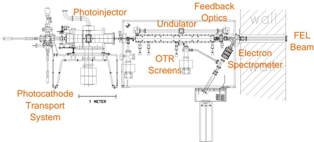
Figure 1. Experimental Layout of the Regenerative Amplifier Free-Electron Laser at Los Alamos.
