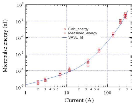
Figure 2: Semi-logarithmic plot of measured SASE micropulse energy versus peak current.
