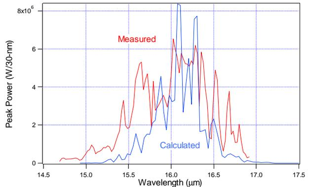
Figure 7: Measured (red) and calculated (blue) infrared spectra of the RAFEL output. The spikes are caused by different co-operation lengths of the high-gain FEL.
