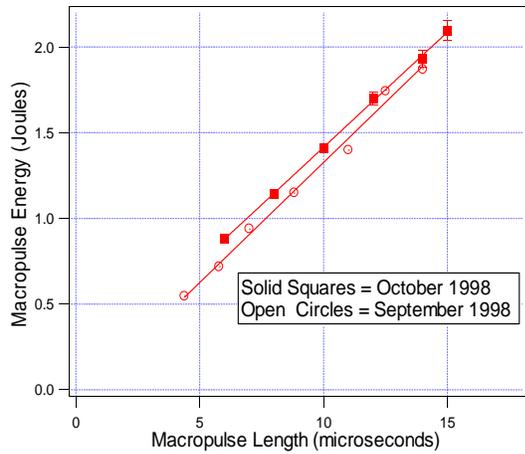
Figure 4: Plots of macropulse energy versus macropulse length. The two different sets of data were collected on different days.
