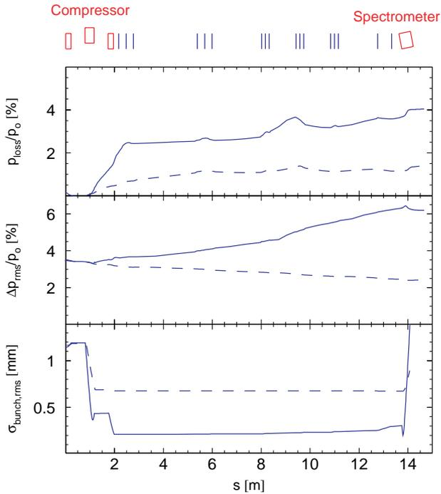
Figure 5: Evolution of the bunch length, the rms momentum spread and the momentum loss (from bottom to top) along the CTF II beam line as simulated with TraFiC<sup>4</sup>, for 10 nC. The results with two different setting of the chicane are shown, corresponding to  $R_{56} = 34$  mm (solid line) and  $R_{56} = 15$  mm (dashed line).
