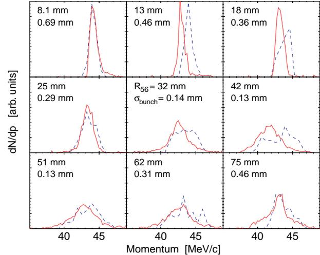
Figure 2: Measured (solid line) and calculated (dotted line) momentum spectra at the end of the beam line for different compressor settings  $R_{56}$ , with a bunch charge of 5 nC. The measured bunch lengths are also shown (lower values).
