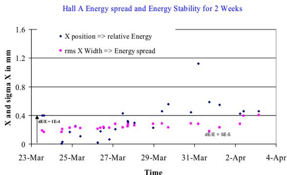
Figure 5: Horizontal position and size of Hall A beam during delivery period. Note the degradation of the spread with time due to uncorrected drifts. Even with drifts, the spread is remarkably small.
