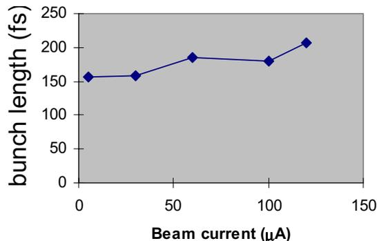
Figure 2: Bunch Length vs. Beam Current out of Injector
