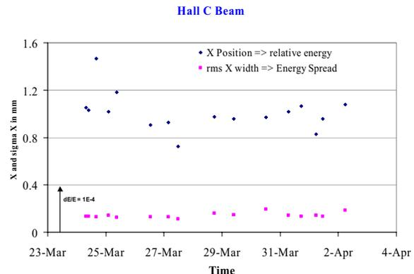
Figure 4: Horizontal position and size of Hall C beam during delivery period. Note that the Hall C beam line provided the energy locking data.
