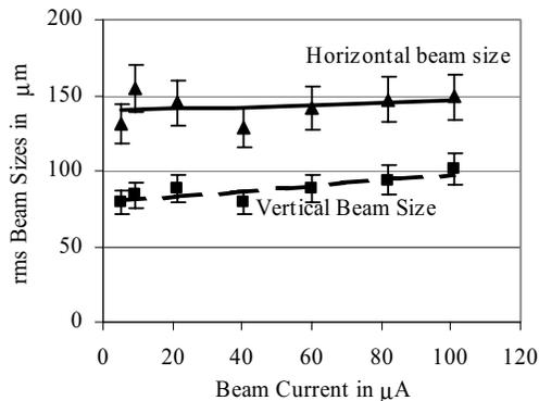
Figure 3: Beam Size vs. Beam Current at high dispersion point in beam delivery line.
