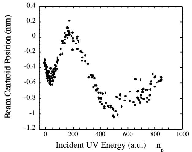
Figure 4: Beam centroid position measured by a beam position monitor located 2.5 m downstream from the plasma exit. This data was acquired at the same time as the beam spot size data shown on Fig. 3.
