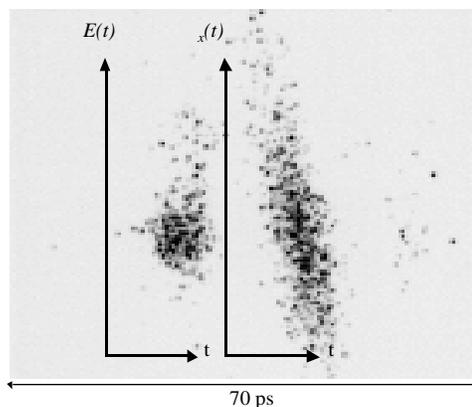
Figure 6: Streak camera image showing the beam energy as a function of time ( $E(t)$ ) on the left hand side, and the beam spot size in the x plane as a function of time ( $x(t)$ ) on the left hand side. Notice the qualitative difference between the 2 streaks. This image was used in the slice analysis shown on Fig. 5.
