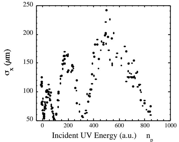
Figure 3: Beam spot size measured at the downstream OTR location as a function of the relative uv laser pulse energy. The plasma density is proportional to the uv energy.
