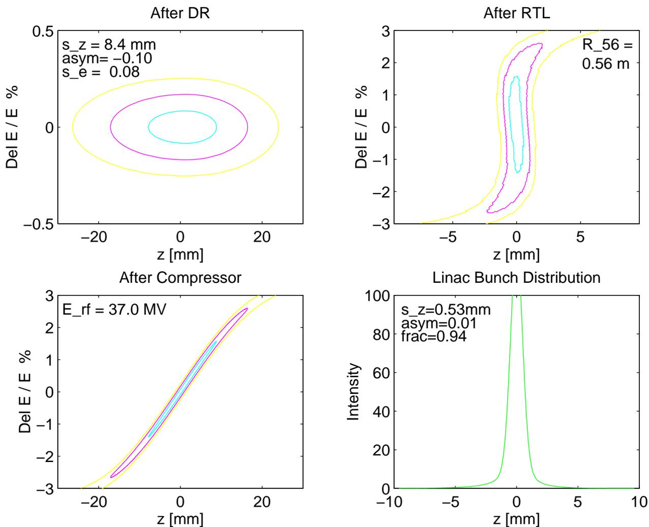
Fig. 2: Bunch length compression in the RTL.
