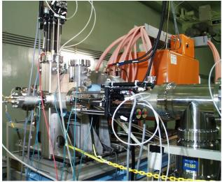
Figure 3: A photograph of the LEBT and beam monitors.
