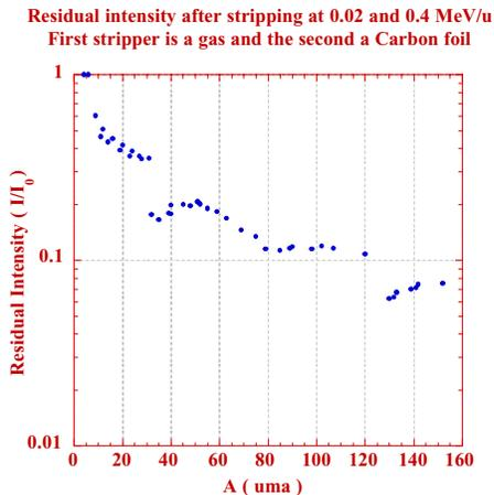
Figure 4: Residual intensity after to strippers. The first stripper is a gas stripper at 0.02 MeV/nucleon and the second stripper is a carbon foil at 0.4 MeV/nucleon.
