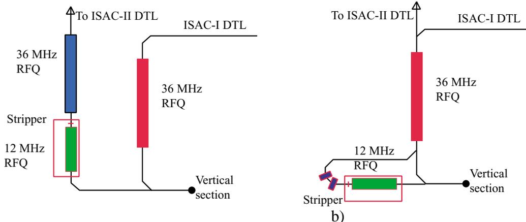
Figure 2: Two schemes using a low frequency RFQ and a gas stripper combination. Figure a represents a
