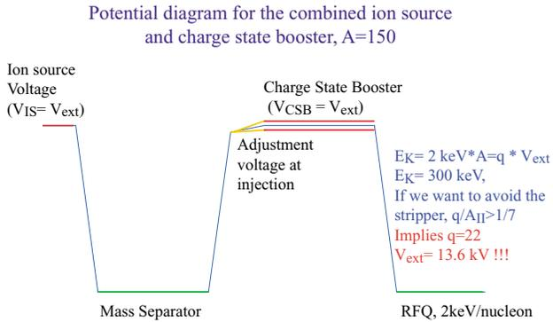
Figure 1: Potential diagram for an ECRIS as charge-state breeder.
