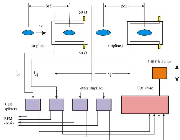
Figure 1. The Energy Spread and Energy Monitor.
