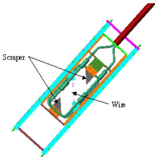
Figure 1: Wire Scanner/Halo Scraper internal measuring axis
