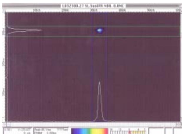
Figure 1: Streak of OTR (Y scale is 400 ns) indicates linac e- beam macropulse length of 8 ns.
