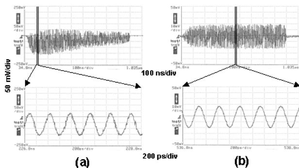
Fig. 7. (a) 2.856-GHz modulated pulsed-waveform for electron beams and (b) input RF waveforms. Top and bottom waveforms are macro and micro pulses, respectively.
