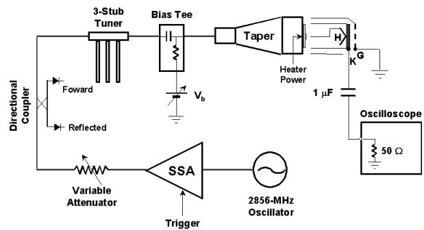
Fig. 2. Schematic diagram of experimental set-up (zero-beam-voltage test) for 2.856-GHz modulation of a conventional triode gun.
