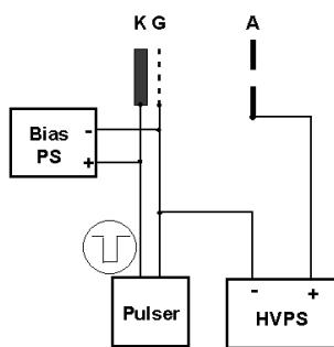
Fig. 1. Schematic diagram for conventional triode gun.
