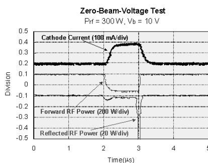
Fig. 4. Typical cathode current and RF powers waveforms
