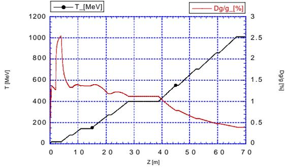
Figure 2: Energy gain and energy spread along the Linac.
