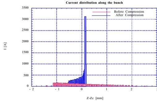
Figure 4: Current distribution along the bunch before (lower curve) and after the magnetic compression.
