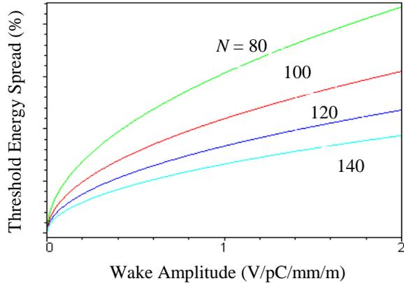
Figure 2: Threshold energy spread  $|f_\gamma|$  (corresponding to  $\eta=1$  at the linac exit) versus deflecting-wake amplitude  $w_0$  and number of betatron periods  $N = 80$  (top), 100, 120, 140 (bottom).
