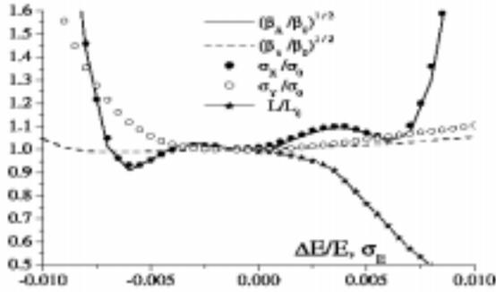
Figure 4a: IP bandwidth of the traditional NLC Final Focus. Normalized beta functions and normalized luminosity equivalent beam sizes Vs energy offset  $\Delta E/E$ , and normalized luminosity Vs rms energy spread  $\sigma_E$ .
