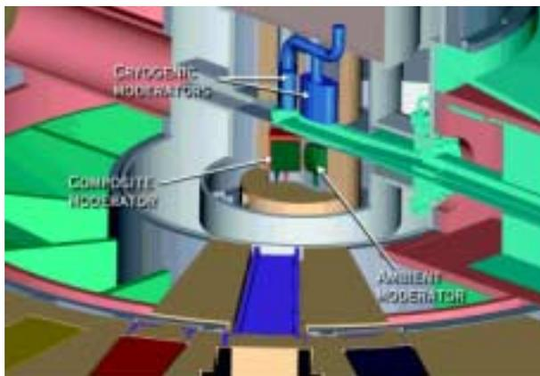
Figure 2: Cross-sectional view of the cryogenic, composite, and ambient moderators and the mercury target. The proton beam arrives from the upper left of the drawing.
