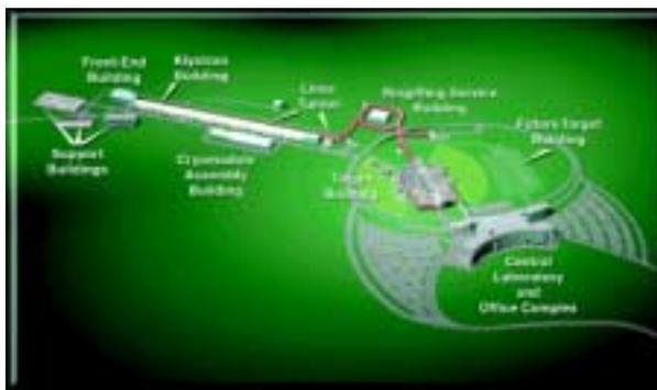
Figure 4: Spallation Neutron Source site plan showing the front end, linac, accumulator ring, target, instruments, and central lab/office and other support facilities.
