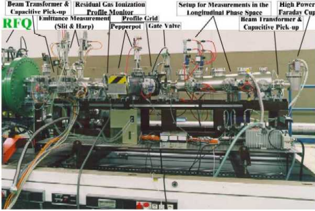
Fig. 3: Beam diagnostic test bench during beam commissioning of the 36 MHz IH-RFQ. [13]
