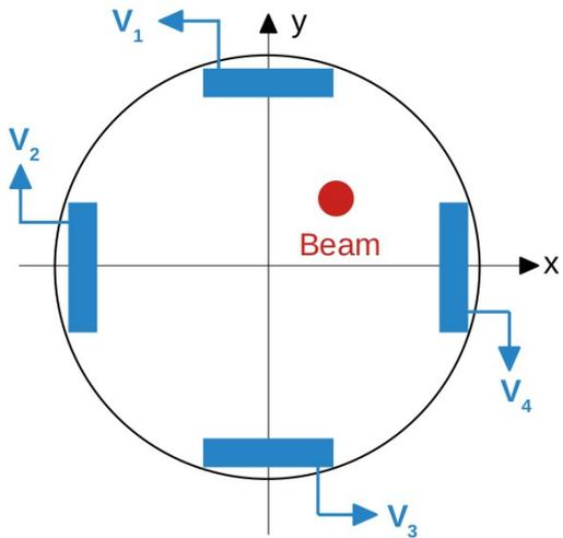
Buttons typically aligned on the transverse axes
