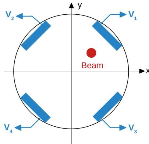
Buttons typically rotated by 45° due to strong synchrotron radiation
