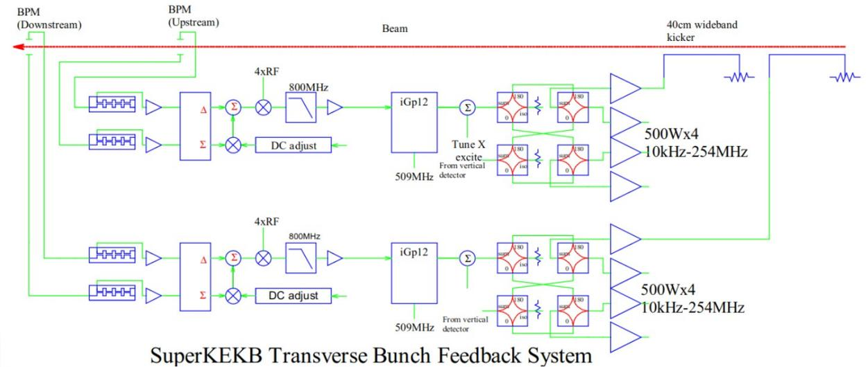
Continuous excitation achieved in SuperKEKB using transverse feedback system and amplification
