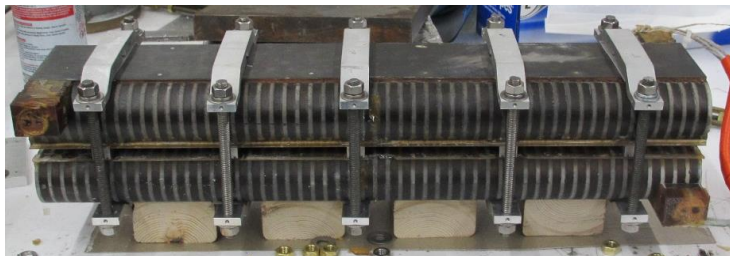
0.5-m-long Nb 3 Sn undulator
